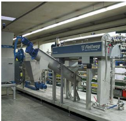
Flottweg Tricanter®-System for low temperature application
