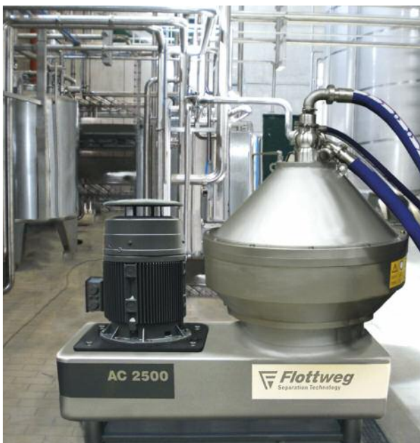
Flottweg Disc Stack Centrifuge AC 2500 for the clarification of fruit juice and fruit wine
