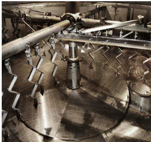
The spent grains: from the straining vat directly onto the belt press
